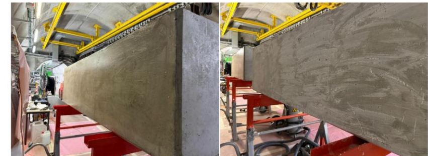
Fix contamination (spray) vs. decontamination (gel) on concrete
