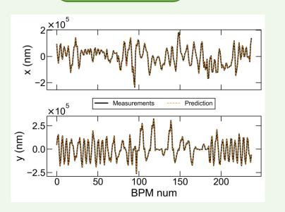
The combined impact of multiple IDs moving at the same time is non-linear. NNs accurately predict the transverse displacement of the beam along the ring for any given ID configuration. Badger/Xopt optimization
