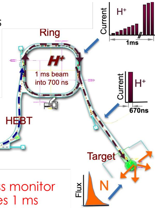
Measured beam losses lead to activation
