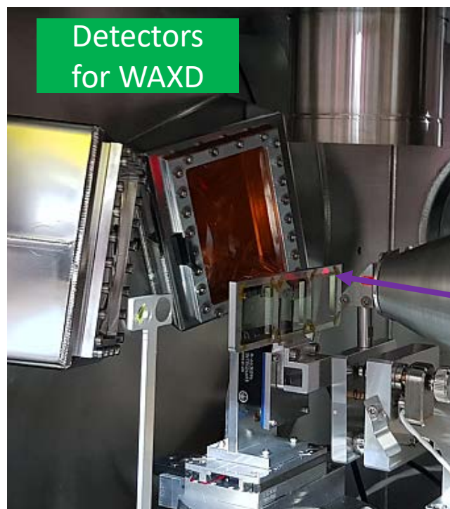
(figure) Pump-probe multiplex imaging using femtosecond X-ray pulses. A femtosecond IR laser drives the melting process of core-shell nanoparticles and small/wide-angle X-ray diffraction patterns are simultaneously collected while changing the time delay of two light sources.
