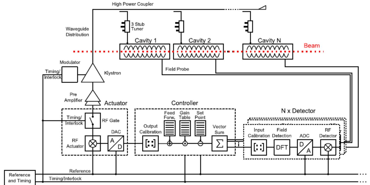
Simplified (old) scheme of a FLASH Accelerating module LLRF system
