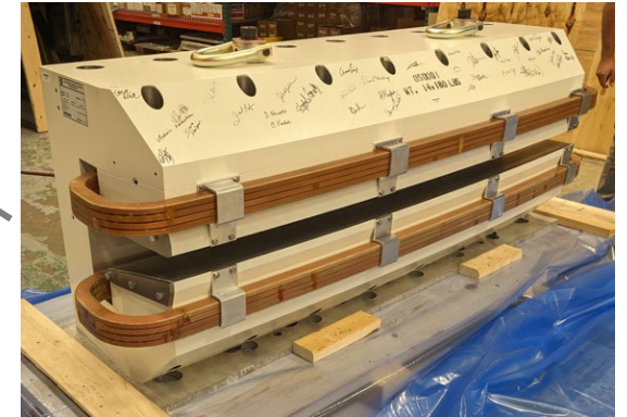
Injection dump dipole ready for installation
