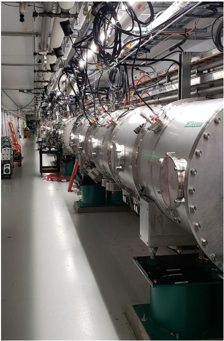
Cryomodules 27 thru 32 installed in the SNS Linac
