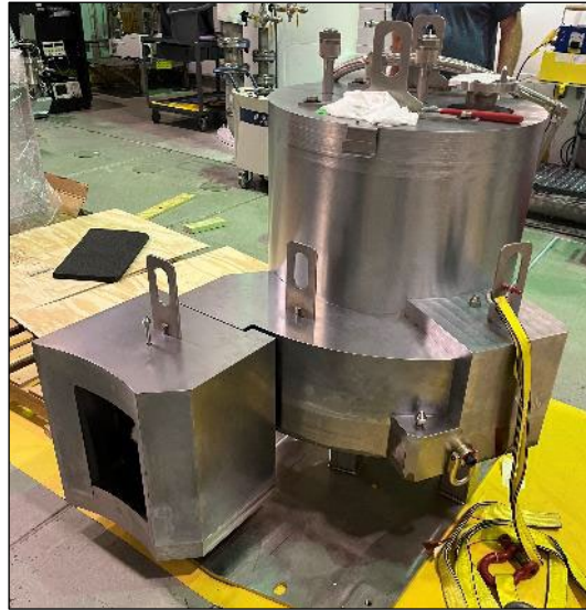
Mercury overflow tank
