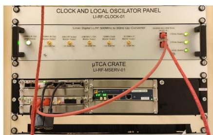
New DLLRF installed in Linac.
