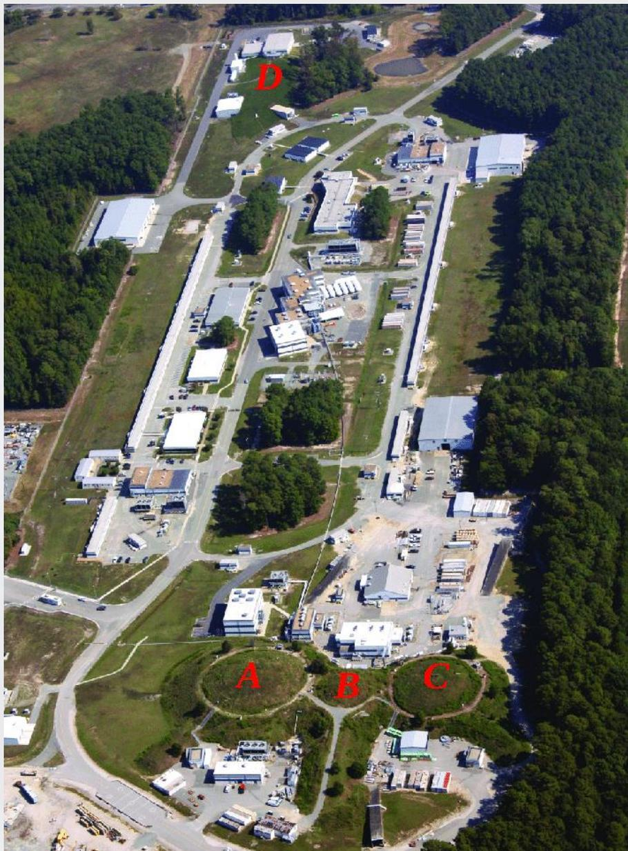
The Continuous Electron Beam Accelerator Facility (CEBAF), at Thomas Jefferson National Accelerator Facility (TJNAF), provides high-quality beams of polarized electrons that allow scientists to extract information on the quark and gluon structure of protons and neutrons. CEBAF operates as a pair of superconducting radio frequency linacs, in a “racetrack” configuration, capable of delivering electron beams simultaneously to four experimental halls.
