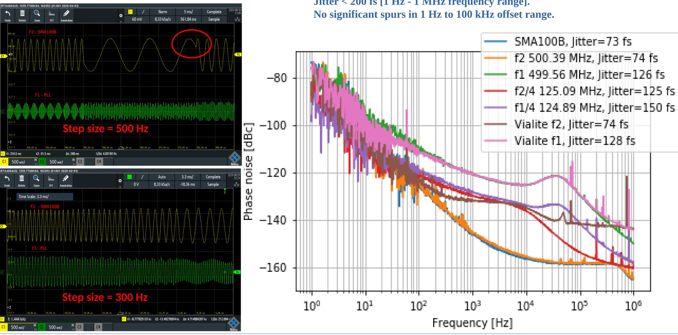
**Measured phase noise and spurs of the new MO system at every output stage:** Jitter < 200 fs [1 Hz - 1 MHz frequency range].
