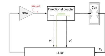
Two causes of  $V_f \neq 0$  (RF off): crosstalk between the measurement channels and source impedance mismatch
