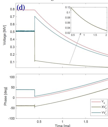
Voltage and phase of cavity signals after turning off the RF power
