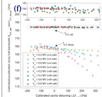
Relationship between the cavity half bandwidth and cavity detuning parameter in the calibrated and uncalibrated algorithms for various values of  $V_c$ .
