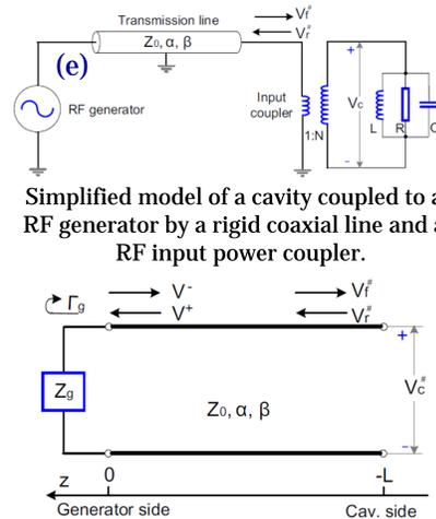
Simplified model of a cavity coupled to an RF generator by a rigid coaxial line and an RF input power coupler.
