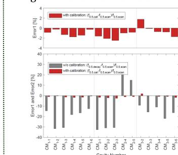
Comparison of the deviation between  $f_{0.5,decay}$  and  $f_{0.5,cali}$  for the 16 cavities and the network analyzer measurement results,  $f_{0.5,scan}$
