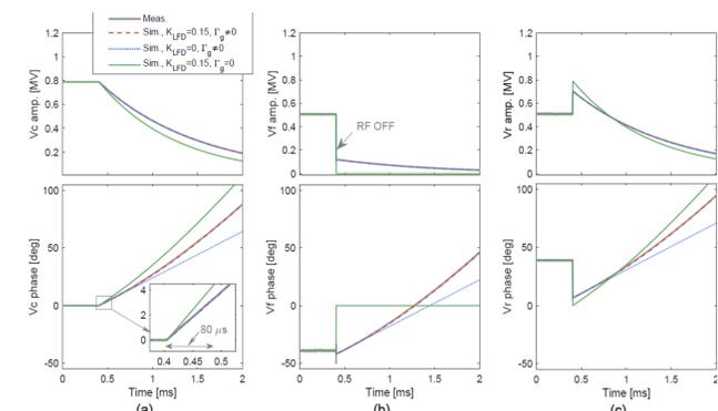
Comparison of the cavity voltage (a), cavity forward (b), and reflected signal (c) measurements based on the cavity model (red) and real SC cavity (gray)
