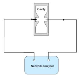
Measurement block diagram based on the network analyzer.
