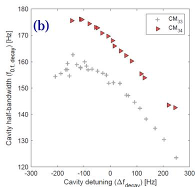
$f_{0.5,decay}$  and  $\Delta f_{decay}$  have dependency relations on cavity CM<sub>3-3</sub> and CM<sub>3-4</sub>
