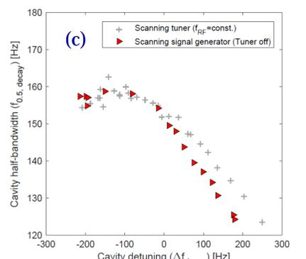
Comparison of the dependency relationships at when  $\Delta f_{decay}$  is scanned by the signal source
