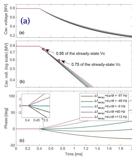
Cavity amplitude and phase decay curves after the RF power is turned off for various  $\Delta f$  on a cavity
