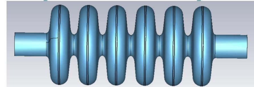
648MHz Elliptical Cavity X 24
