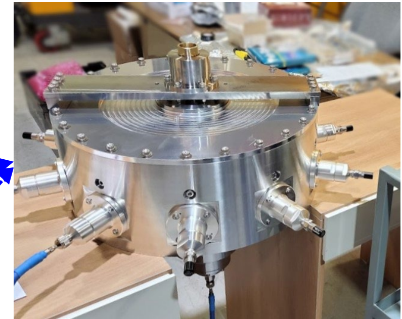
10 way cavity combiner for the SSPA
