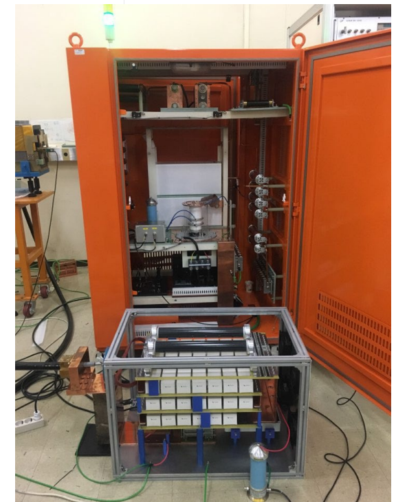
Solid-state switch test in PLS-II
