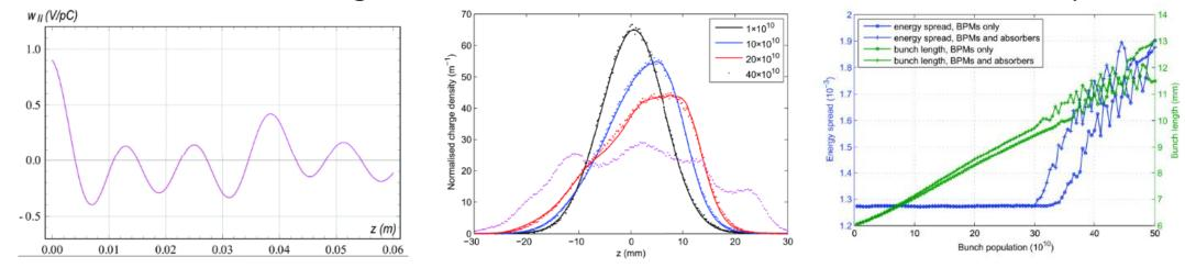
The solutions to the Haissinski equation (solid lines in center plot) can be compared with the results from particle tracking (dots). At high bunch charges, no equilibrium solution exists: the bunch is unstable.
