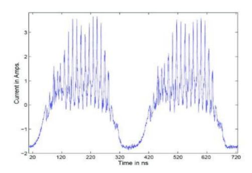
Observation of single-bunch longitudinal instability in the Los Alamos PSR, caused by an inductive impedance.
