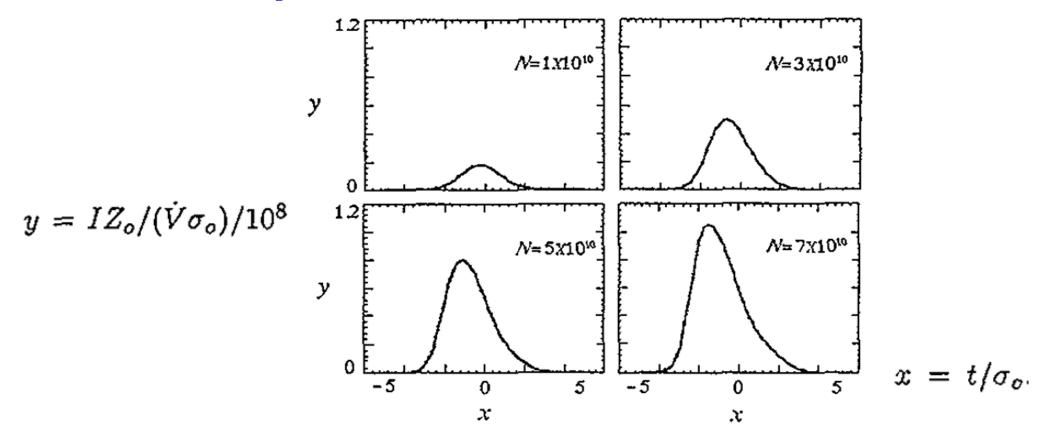
Calculated bunch distribution due to potential well distortion for various beam intensities in KEK-ATF damping ring
