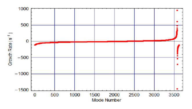
(growth rate *vs* mode number for the resistive wall wake) Roughly half the modes grow (are unstable), and half the modes are damped.
