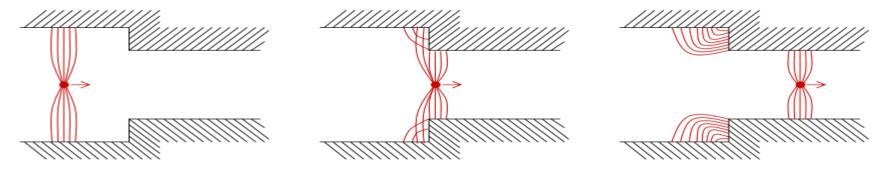
■ Under some conditions, the perturbation on the beam are continously enhanced by the wakefield, leading to the collective instabilities.
