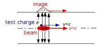
Ultrarelativistic beam going down perfectly conducting smooth vacuum pipe
