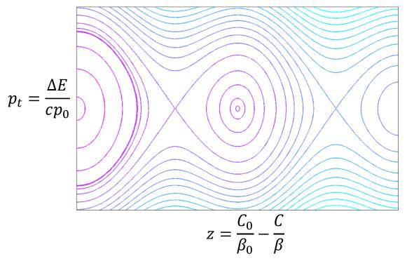
Note that there are bounded regions where the contours form closed loops: particles in these regions perform stable oscillations. The curve forming the boundary of stable region is called the separatrix.
