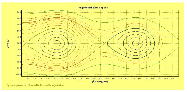
$$E = 3.0~GeV, V_{RF} = 3.2~MV, f_{RF} = 499.97323~MHz, h = 470, U_0 = 1.04~MeV$$
