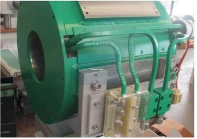
• Insertion devices (IDs) consisting of sequences of (short) dipole magnets of alternating polarity are used in light sources to enhance the production of synchrotron radiation
