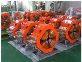
Other kinds of magnet are used for more refined control over the beam properties: sextupole, octupole, corrector (a few hundred Gauss), skew-quadrupole magnets etc.
