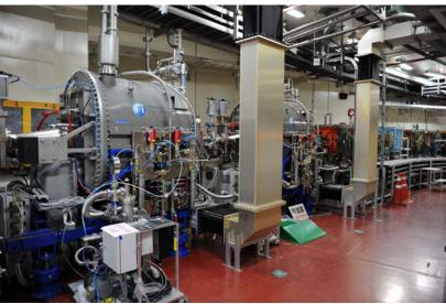
However, at high field strengths, the amount of power dissipated in the walls of the cavity through induced electrical currents can be considerable, and it is usually necessary to provide cooling, by means of water flowing through pipes or channels fitted around the cavity.
