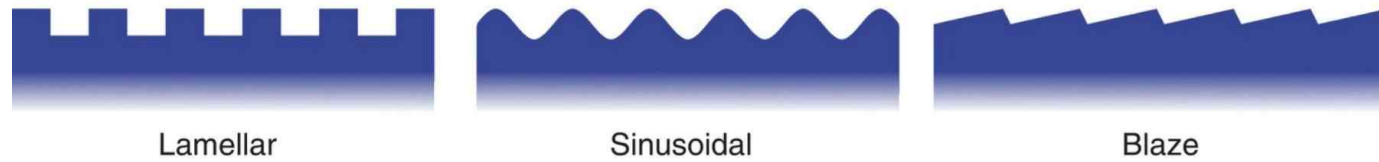
Figure 5.21 Three common grating profiles used to disperse ultraviolet light and soft x-rays.
