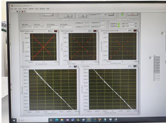
Figure 5: A position control system of the translation stage displayed on the data acquisition computer.
