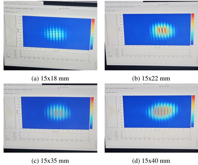
Figure 6: Interference pattern observed in the beamline depending on the size of double slits.
