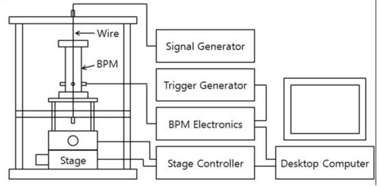
Figure 3: The wire test stand for the position sensitivity and the offset measurement in a nutshell [1].
