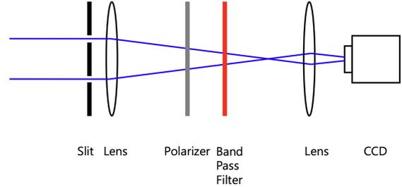
Figure 4: A schematic layout of the SR interferometer apparatus.
