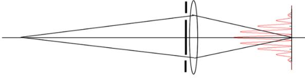
Figure 2: A simple representation of the visibility of an interferogram and light source size [2].
