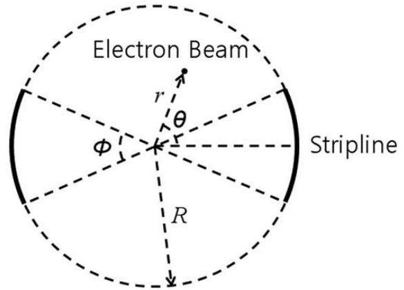
Figure 1: A transverse drawing of a typical stripline BPM.
