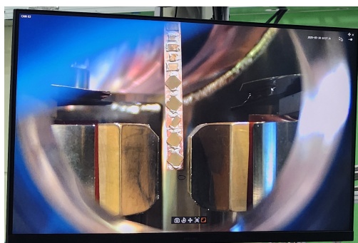
(a) A series of sample fragments are inserted to the beam core.
