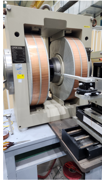
Figure 3: A dipole electromagnet model 3474-140 manufactured by GMW Association.
