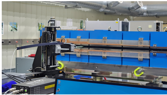
Figure 2: An overview of the Hall sensor and electromagnet. The tip of the sensor measures the magnetic field by scanning between two magnets.
