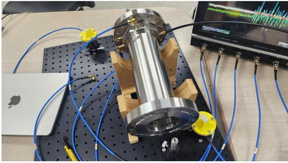
Figure 3: Pickup type BPM sensors measuring the signal of conducting wire and TDR is employed together.
