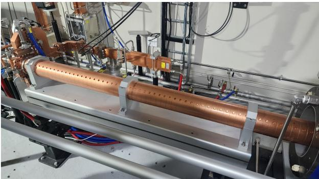
(b) RF cavity for the particle to be accelerated
