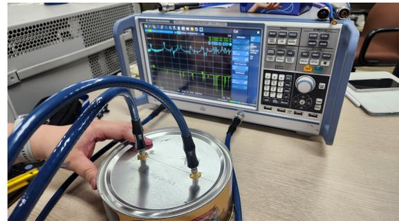
Figure 2: S-parameters of the pillbox cavity is measured by the VNA which displays the parametric graph.
