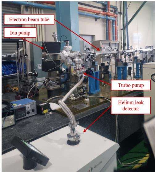
Figure 2: Prototype of electron beam tube and vacuum system.
