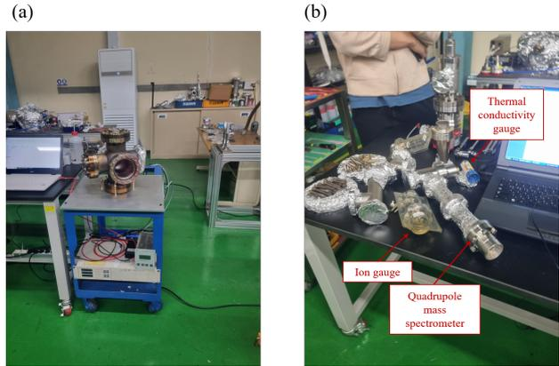
Figure 3: (a) Picture of vacuum chamber before disassembly. (b) Gauges prepared for integration onto the vacuum system.
