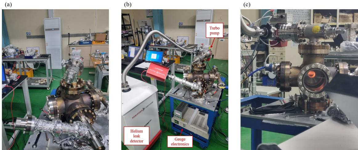
Figure 4: (a) Vacuum chamber after the installation of gauges. (b) Connection of helium leak detector and gauge electronics which measure and display the pressure inside the chamber. (c) Another view of vacuum chamber showing the interior through a window.
