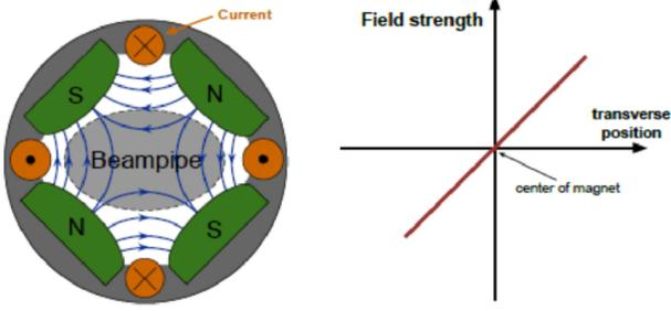
Figure 2: The basic structure of normal quadrupole magnet. The magnetic field strength increases linearly with the transverse position.
