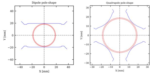
Figure 3: Transformation of a dipole-like structure into a quadrupole-like structure through the conformal mapping  $w = z^2$ .
