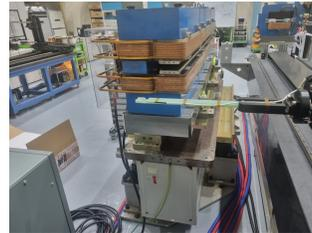
Figure 5: Hall probe system and the bending magnet used for magnetic field measurement. The Hall probe scans along the beam trajectory to measure the field profile.
