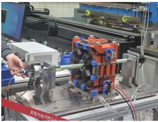
Figure 4: The rotating coil setup used in the experiment. A coil is placed inside the quadrupole magnet and rotated to measure the magnetic field.
