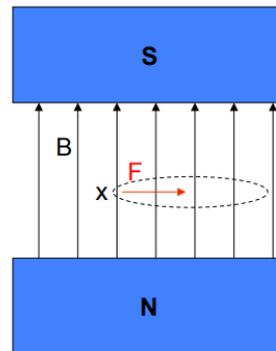
Figure 1: Basic structure of normal dipole magnet. The magnetic field strength is uniform across the magnet.
