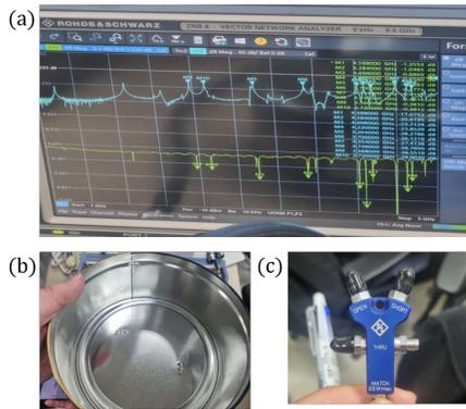
Figure 3: Devices of the VNA experiments: (a) vector network analyzer, (b) pillbox cavity, (c) calibration kit.
