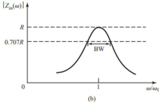
Figure 1: Impedance of a cavity modeled as a parallel RLC circuit [1].
