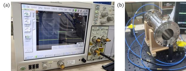
Figure 4: TDR measurement setup with BPM: (a) TDR devices, (b) stripline BPM.
