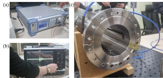
Figure 5: Experimental setup for BPM signal measurement: (a) signal generator, (b) oscilloscope, (C) wire inside BPM.
