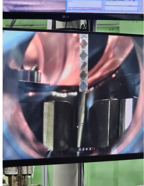
Figure 2: Sample stage of 2A-beamline: By adjusting the magnets placed on either side of the sample, the effective polarization of the incident light interacting with the sample can be controlled
