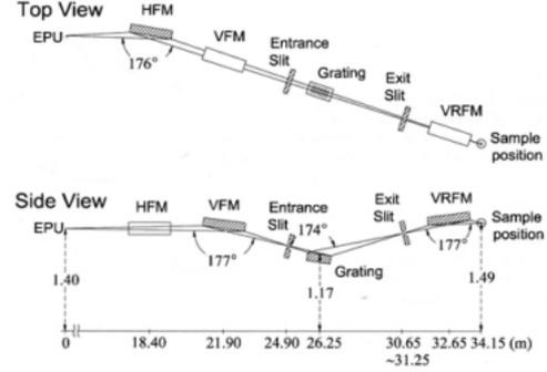
Figure 1: Schematic view of PLS-2 beamline
