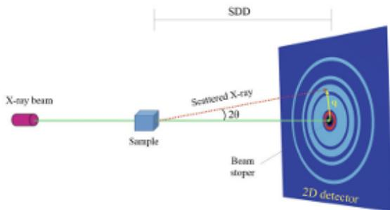
Figure 1: Schematic of the SAXS experimental setup showing the X-ray beam, sample stage, and 2D detector.
