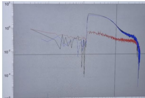
Figure 4: Scattering profile of BSA measured in flow mode. Red: subtracted result, Blue: background, Black: raw intensity.
