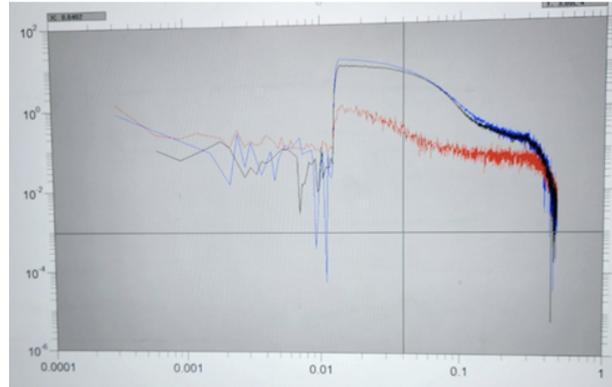
Figure 3: Scattering profile of BSA measured in static mode. Blue: BSA in water, Black: solvent, Red: subtracted profile.
