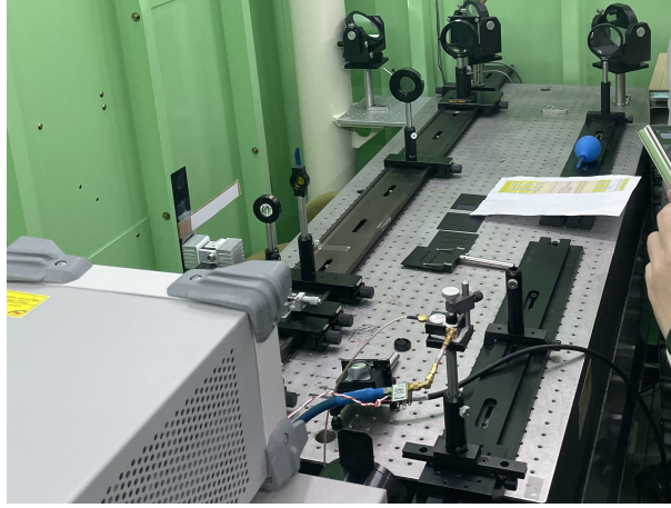
Figure 2: Schematic of Synchrotron Radiation Interferometer at 1B beamline
