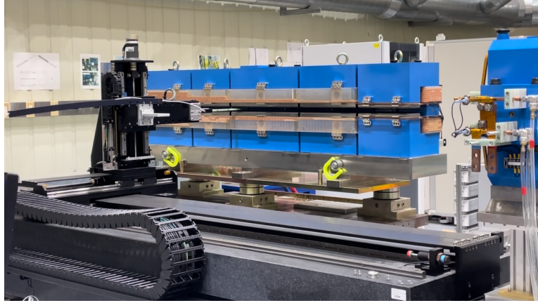
Figure 1: Experimental setup for measuring magnetic fields using a Hall sensor.
