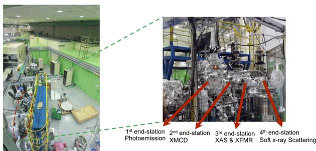
Figure 2: Schematic diagram of the experimental setup at the 2A EPU beamline [2].
