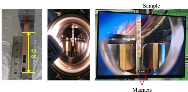
Figure 3: Sample preparation and mounting for XAS and XMCD measurements. (Left) Sample attachment process for preparing thin-film samples [2]. (Center) Inserting the fabricated sample into the vacuum chamber [2]. (Right) Sample holder positioned inside the measurement area, monitored by a camera.
